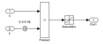
You can also constrain signals that are intermediate or output values of the model. Constraining such signals makes it easier to work around multiplication or division inside lower level subsystems that do not depend on model inputs.
