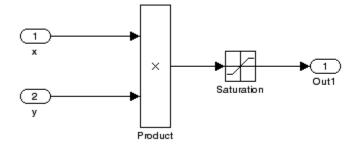
The Simulink Design Verifier software generates errors when attempting to satisfy the upper and lower limits of the Saturation block, because the software does not support nonlinear arithmetic. To work around these errors, restrict one of the inputs to a set of discrete values.
