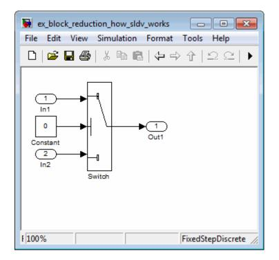
For this Switch block, the control input is always 0. If the **Criteria for passing first input** block parameter is  $u_2 \sim = 0$ , the Switch block always passes the third input through to the output port. When you analyze this
