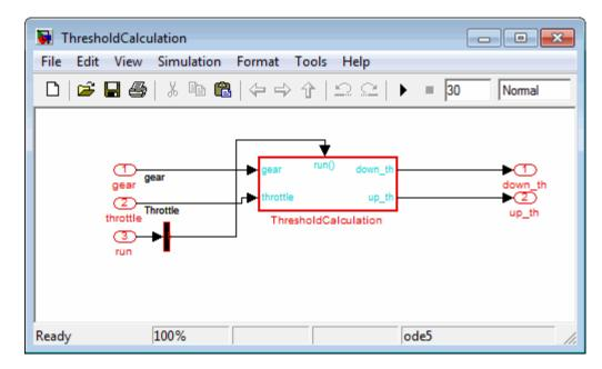
The Inport block and the new subsystem block mimic the trigger for the function-call subsystem ThresholdCalculation in the new ThresholdCalculation model.
