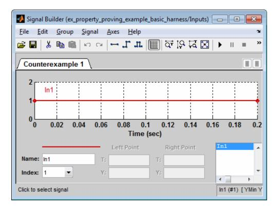
The input signal 1 causes the output of the Compare to Zero block to be 0. This counterexample violates the proof objective that specifies that the output of the Compare to Zero block be 1.
