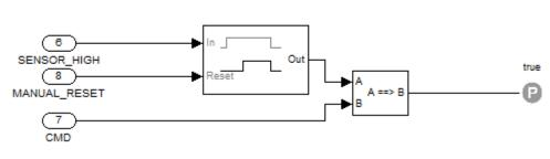
After Sensor is detected at HIGH for 5 consecutive steps, Cmd becomes and stays true for the remaining duration of the Sensor value HIGH unless manual reset is detected.
