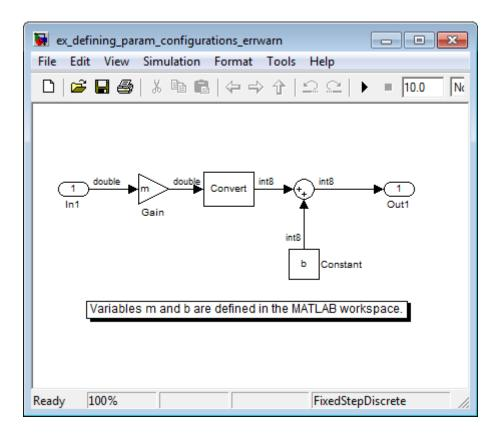
The  $\tt PreLoadFcn$  callback function defines m and b in the MATLAB workspace when you open the model:
