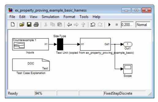
**3** In your harness model window, connect the output signal of the Test Unit subsystem to the Scope block.
