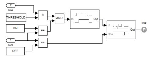
Whenever In3 is ON and In4 is less that THRESHOLD, then In3 shall become OFF within 5 steps.
