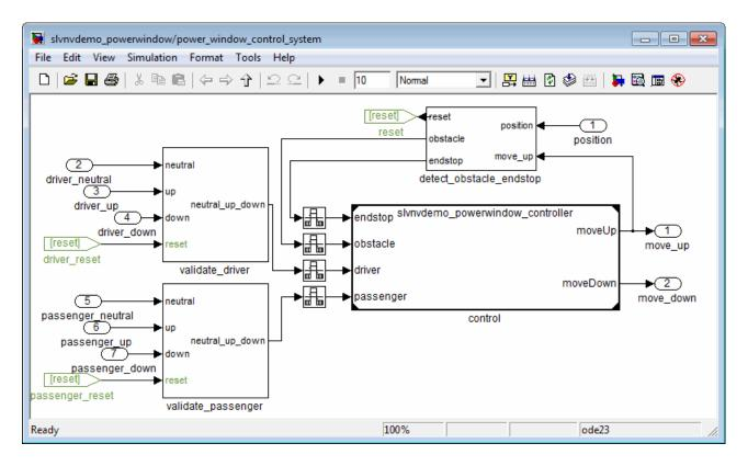
The Model block references the slvnvdemo\_powerwindow\_controller model.
