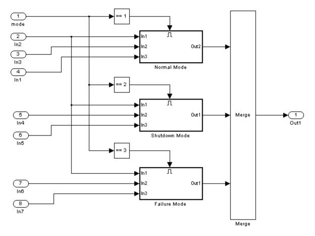
You can incrementally generate test cases for each subsystem by constraining the first input to the appropriate constant value before running an analysis. In this way, as you create test cases for each subsystem, the software ignores the complexity of the other two subsystems.
