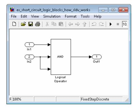
When the Simulink Design Verifier software analyzes this model for Condition Decision coverage, the analysis can only satisfy five of six objectives for the Logical Operator block inputs. The software cannot generate a test case for when the third input to the Logical Operator block is false. If the second input is false, the third input is false, but the software ignores the third input due to the short-circuiting. If the second input is true, the third input is never false.
