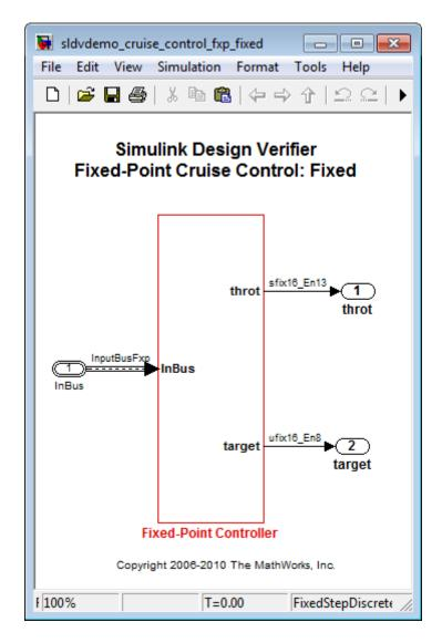
When the analysis is complete, the Simulink Design Verifier Results window initially displays a summary of the analysis results. The analysis detected design errors in four objects in the sldvdemo\_cruise\_control\_fxp\_fixed model. The analysis also identified test cases containing signals that generate those errors.
