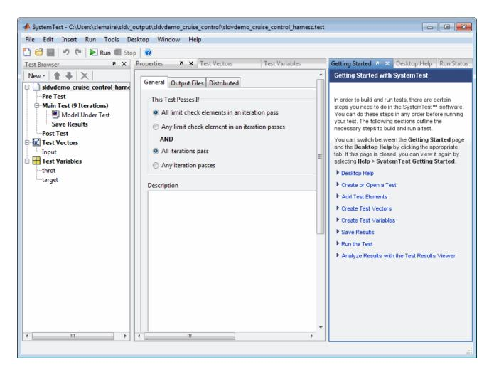
In the **Test Browser** pane, the 9 iterations under Main Test correspond to the 9 test cases the Simulink Design Verifier software generates and describes in the Test Case Explanation block of the harness model.
