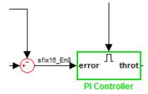
This Sum block can produce an overflow error. The analysis found a test case that can result in a computation where the output of the Sum block exceeds the range  $[-128\ 128]$ .
