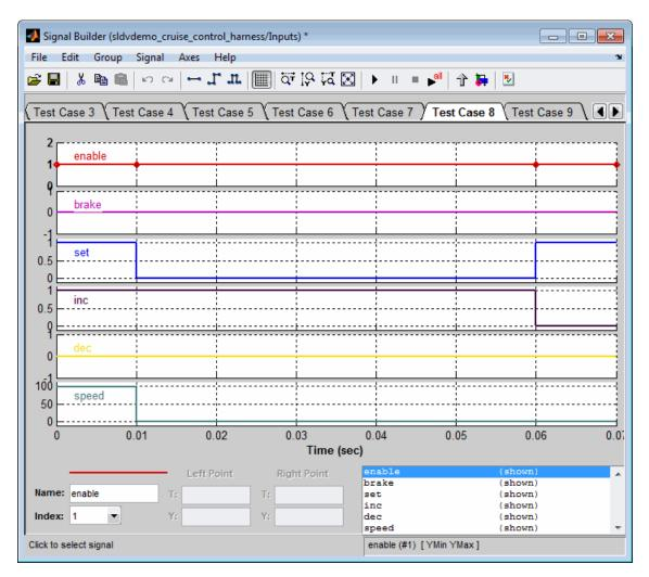
If you select the LongTestcases option of the **Test suite optimization** parameter, the analysis creates fewer, longer test cases. For example, if you select the LongTestcases option for the sldvdemo\_cruise\_control model, the analysis produces one long test cases instead of nine shorter test cases. The following Signal Builder dialog box shows the signals for one of those two test cases.
