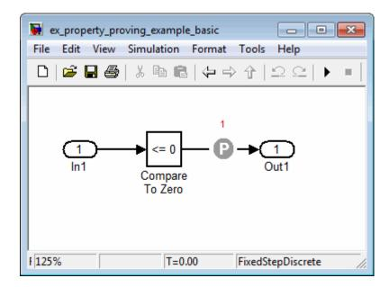
The Proof Objective block is highlighted in red, which indicates that a proof objective was falsified with a counterexample.
