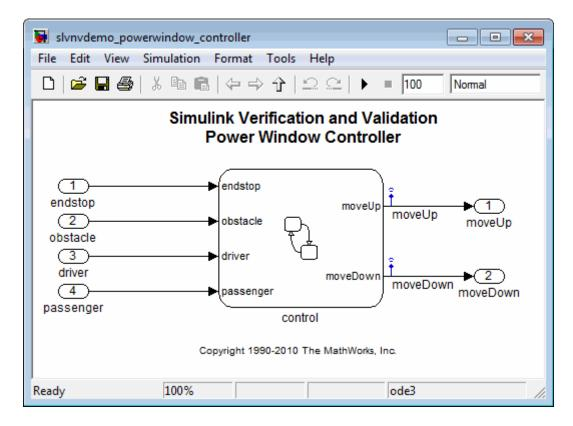
The referenced model contains a Stateflow chart control, which implements the logic for the power window controller.
