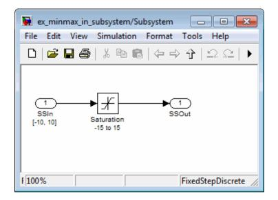
In Subsystem, the specified minimum and maximum values for input port SSIn are -10 and 10, respectively. The lower and upper limits for the Saturation block are -15 and 15, respectively.
