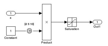
• When you work with large models that have many multiplication and division operations, you may find it easier to add constraints to all of the floating-point inputs rather than to identify the precise set of inputs that require constraints.
